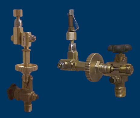
Do not need to change existing filling hoses or filling connectors. Connect the Double Swivel between the hose and the connector. This enables you to fill bottles with top or side outlet cylinder valves. The rotation is around the axial and vertical axes.
